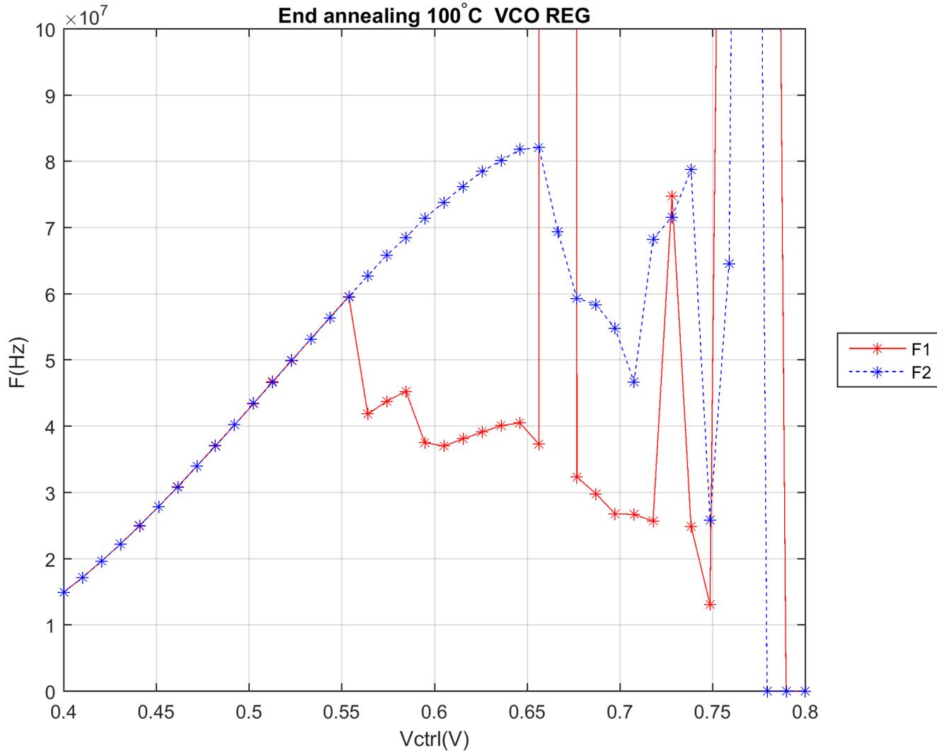
2. Vctrl sweep for ELT transistors VCO (measuring the frequency vs Vctrl).
